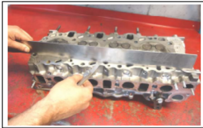
Using a Straight Edge with a Feeler Gauge to measure warp on a cylinder head.
