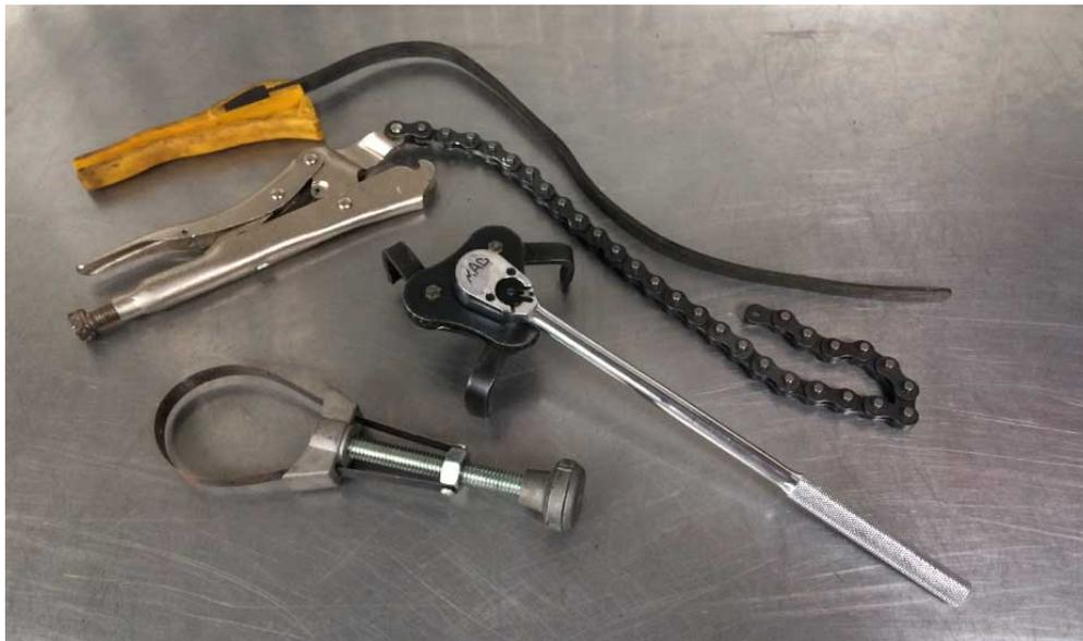
Older style car oil filters are a simple metal filter that screws onto an oil filter adaptor on the side of the engine block. Although oil filters are only fitted hand tight (oil filter tools are not needed for fitting), the filters do tight over time and so a tool is needed to remove them.
