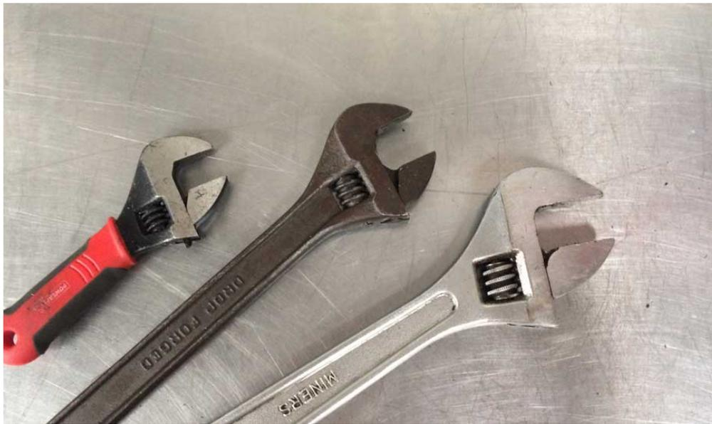
The adjustable wrench is a tool box staple, it's especially popular with plumbers. Not a tool I would use very often, a mechanic will prefer to have a more precise wrench fit, the adjustable wrench, although very flexible, can be a little cumbersome to use.
