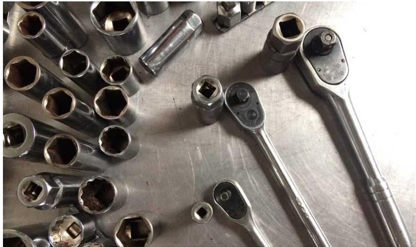
A ratchet is a tool used to drive sockets. It is much faster loosening and tightening fasteners than a spanner, however it is a lot bulkier.
