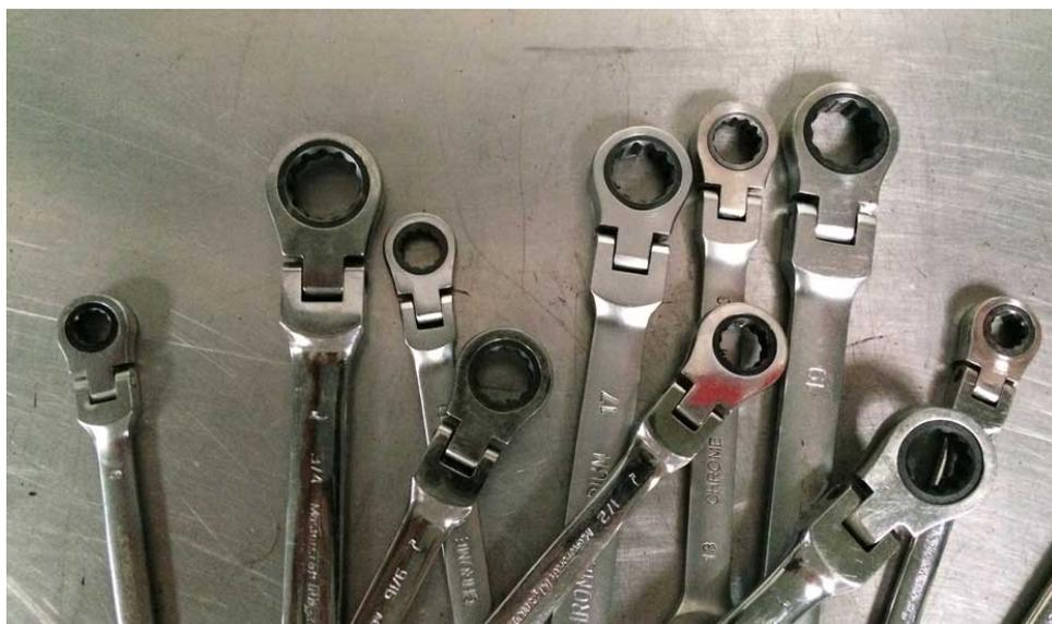
Wrenches are precision tools, each one is a fixed size and will only fit its corresponding nut or bolt size. Commonly made using industrial-grade chromium-vanadium steel.
