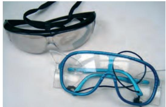
Eye protection that is used to guard against the threat created by flying objects should include lenses that are of the high-impact resistant type.
