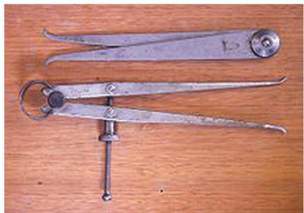
*Fig. 4.3: Outside callipers Fig. 4.4: Inside callipers*
