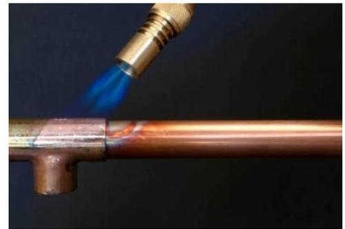
The melting point of parent metal should be higher than filler metal. Mechanical strength of brazed joint is low compared to other joints. This type of joint is suitable in moderate range of temperature areas.
