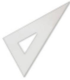
The one problem with an isometric sketch arises when pipes are on angles other than horizontal or vertical; such as 45 degree fittings. These "odd" angles are drawn as they would appear using 60 degree angles. When trying to draw circles in isometric drawings you will have to use an ellipse. A simple drawing tool called a triangle with the angles 30-60-90 will help you keep your drawing in the proper perspective. You can also purchase isometric graph paper or use printable graph paper.
