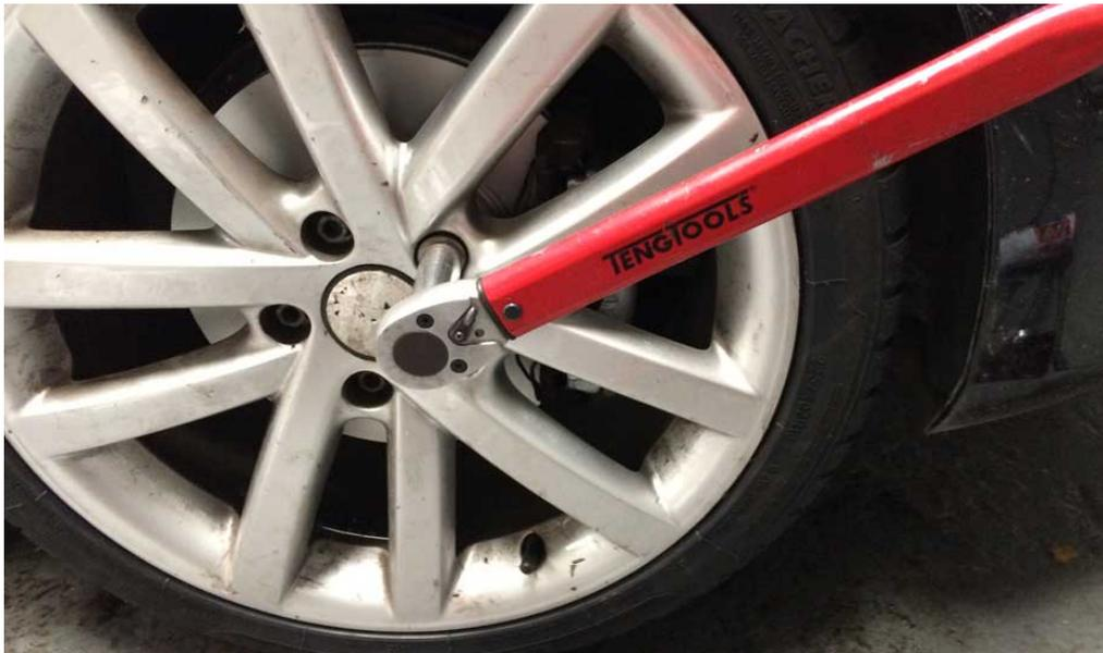
A torque wrench is also needed when replacing a water pump, front engine cover, camshaft cover, oil pan etc. Over-tightening these components can lead to oil leaks and serious engine damage.
