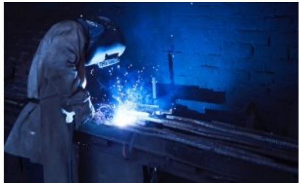
These welders can utilize either DC otherwise AC, & electrodes like consumable otherwise non-consumable. Generally, the welding location can be defended with some kind of shielding gas, slag, otherwise, vapor. This welding process could be manual, fully, or semi-automated.
