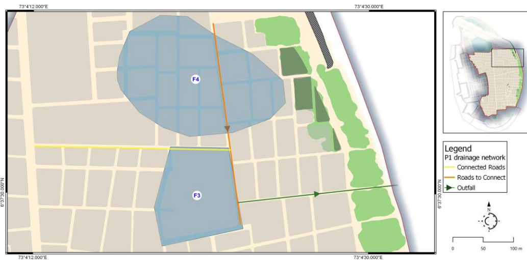
Figure 15: Gravity outfall mechanism proposed for existing aquacells
