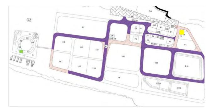
Figure 1. Proposed location of fuel tanks (yellow highlight), septic tank (green highlight) and road connections (red hatch). The purple hatch shows roads proposed in earlier reports
