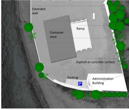
Figure 6: Concept layout design of the transfer station<sup>24</sup>
