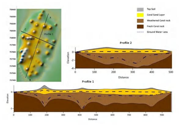
Figure 4-2: Geological sections of the island showing subsurface geological characteristics
