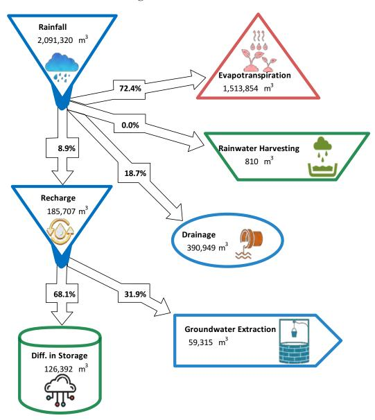
Figure 7-21: Schematic of water balance in Molhadhoo Island
