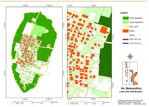
Figure 4-17: Roof Cover in Maarandhoo Island based on UAV Survey
