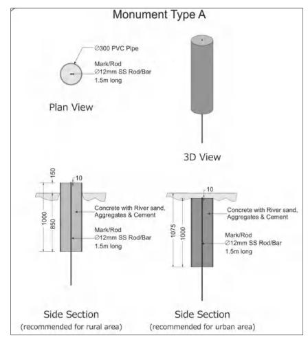
Figure 1-5: Type A PSM design (Source: Maldives Land and Survey Authority, Guideline on the Establishment of Permanent Survey Marks)
