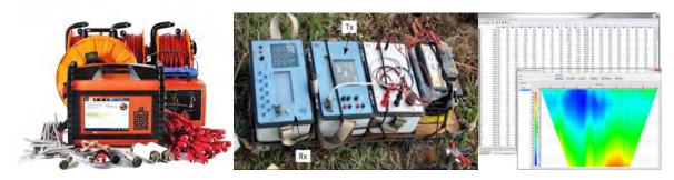
Figure 1-4: Electrical Resistivity (ER) equipment used for the field pilot tests (Sources: Left - ABEM Terrameter LS 2 - User Manual, 2017/ Center, Right - Siqueira Neto & Elis)
