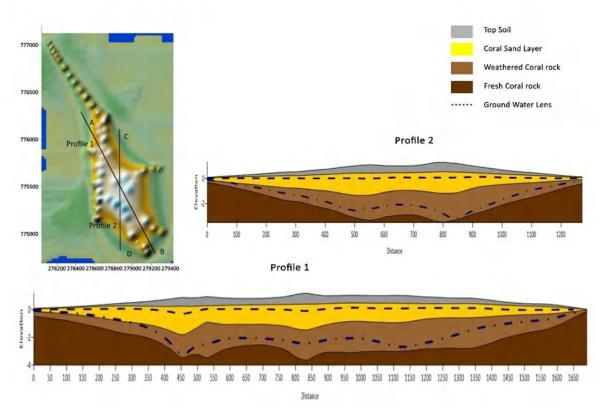
Figure 7-2: Geological sections of the island showing subsurface geological characteristics
