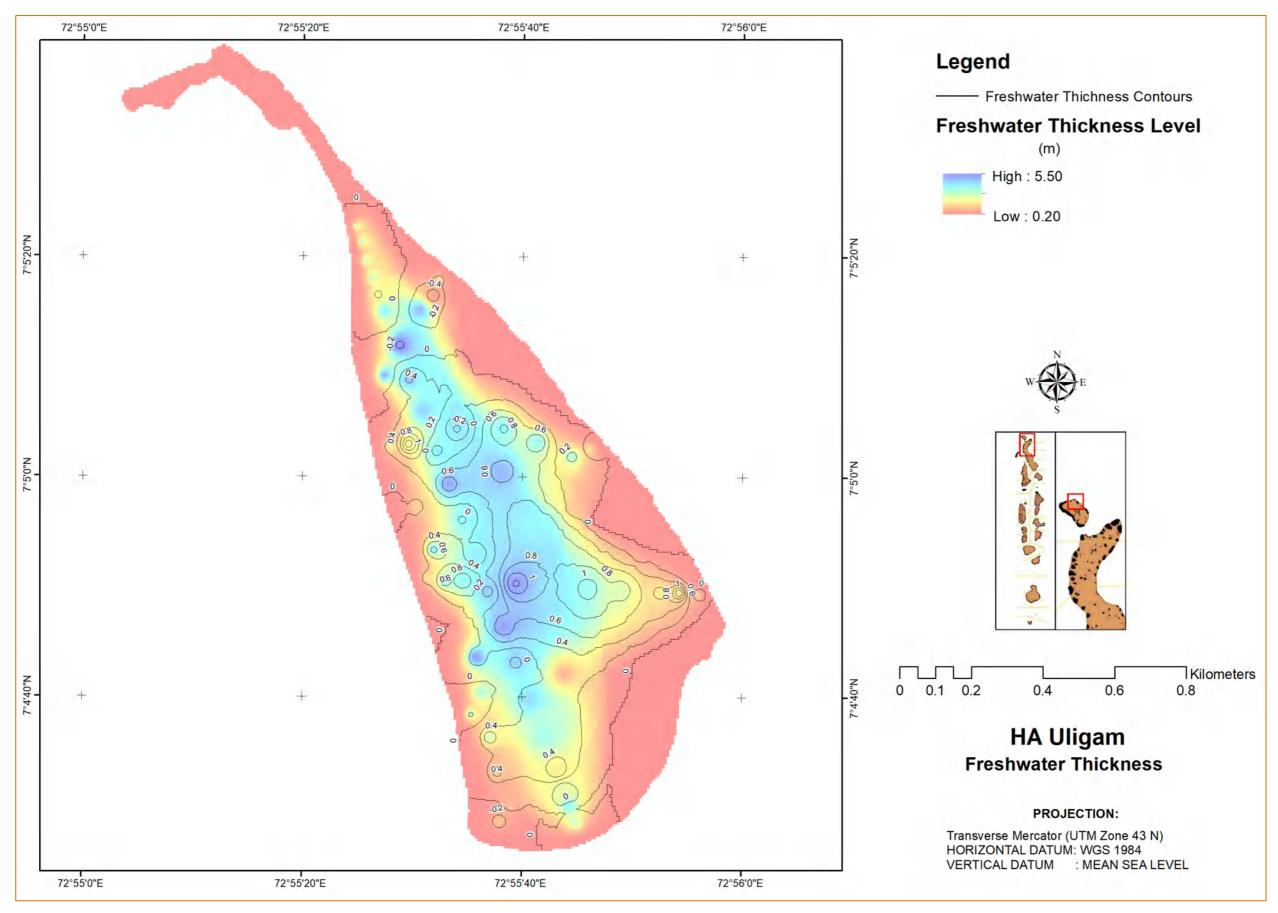
Figure 6-20: Freshwater thickness in Uligan Island
