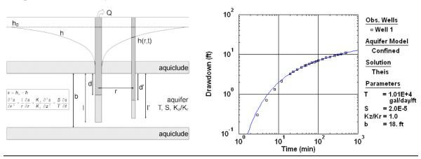
Figure 1-11: Typical well configuration for pumping test in nonleaky confined aquifer and Estimation of aquifer properties by matching Theis (1935) type-curve solution to time-drawdown data
