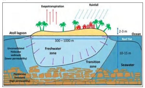
Figure 2-1: Cross section through a small coral island showing main features of a freshwater lens (exaggerated vertical scale) (Source: Jaleel et al., 2020)
