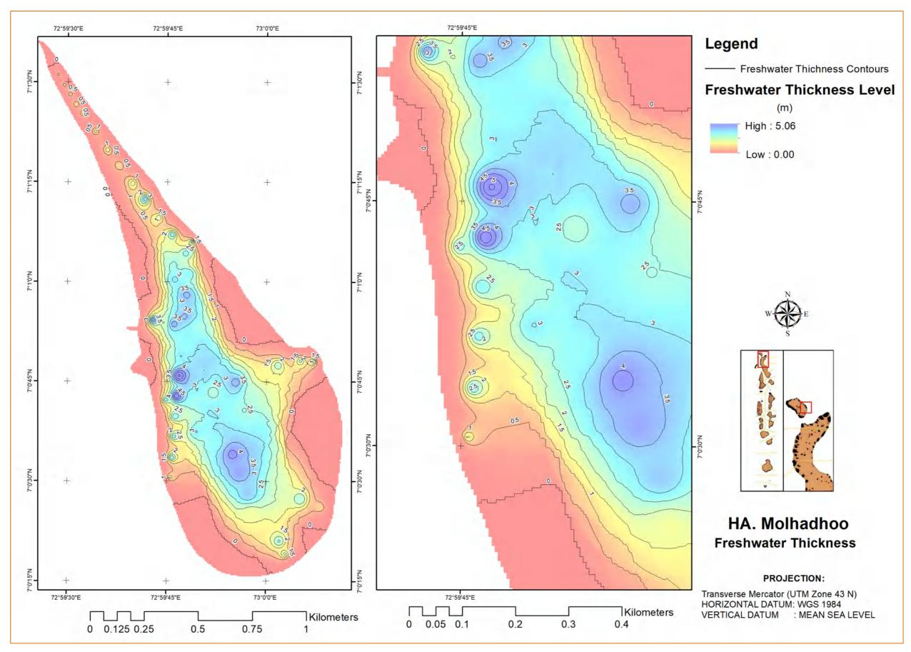
Figure 7-20: Freshwater thickness in Molhadhoo Island
