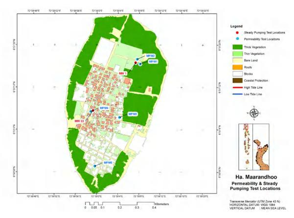
Figure 4-22: Locations of permeability and steady pumping tests in Maarandhoo Island
