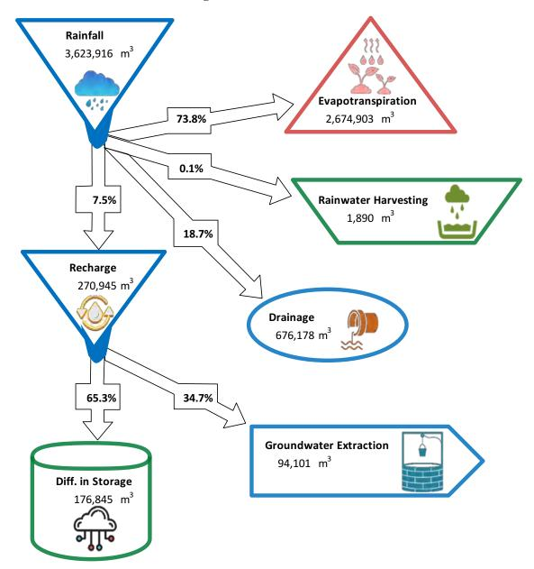
Figure 3-21: Schematic of water balance in Filladhoo Island
