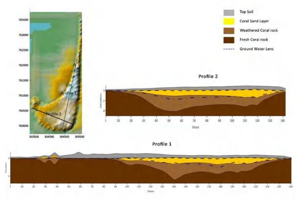
Figure 3-2: Geological sections of the island showing subsurface geological characteristics
