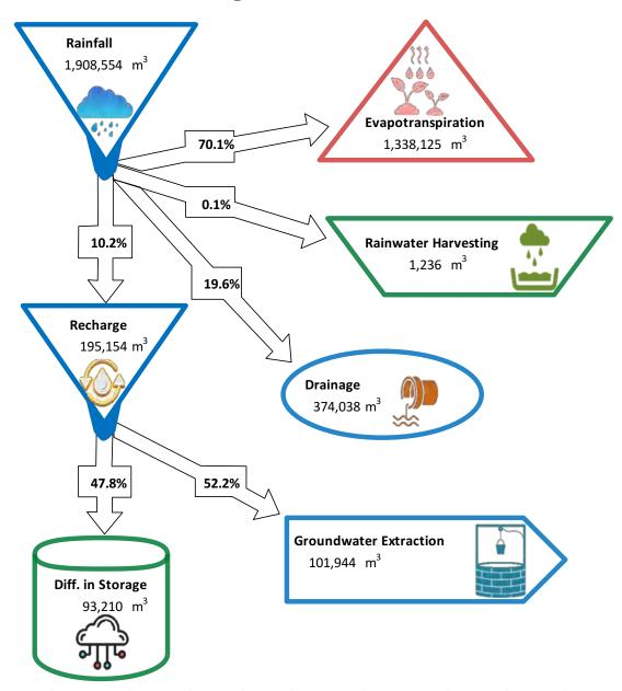
Figure 6-21: Schematic of water balance in Uligan Island
