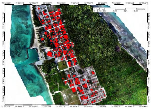
Figure 1-9: Calculation of Roof Cover in an island using UAV survey in the Maldives (Ha. Uligan)
