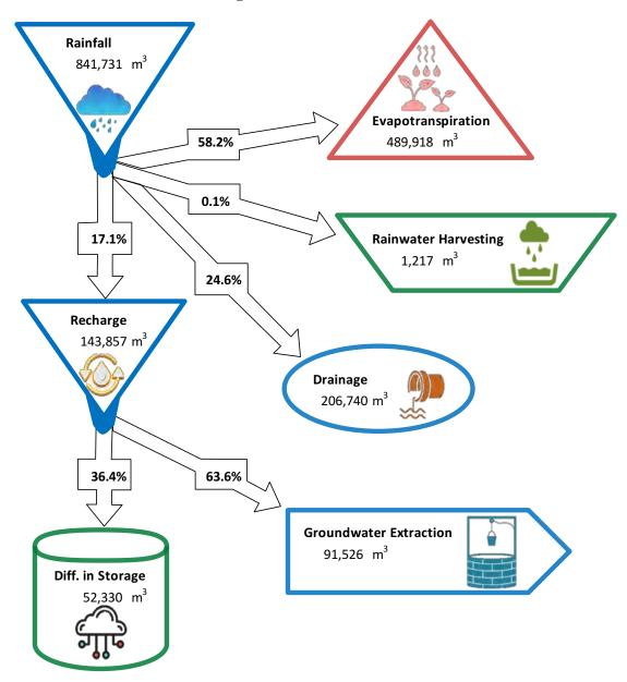
Figure 5-20: Schematic of water balance in Muraidhoo Island
