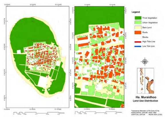
Figure 5-16: Roof Cover in Muraidhoo Island based on UAV Survey
