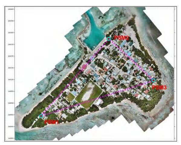
Figure 1-7: Example of spacing of PSMs
