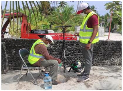
Figure 1-10: Methodology for Constant Head Gravity Permeability Tests
