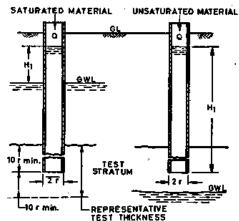
The permeability by constant head method (open-end test) should be obtained from the following relation determined by electrical analogy experiments:
