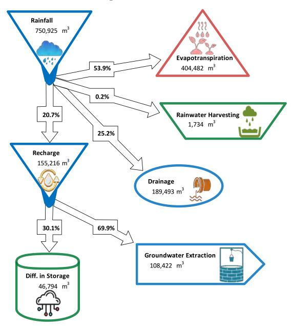
Figure 4-21: Schematic of water balance in Maarandhoo Island
