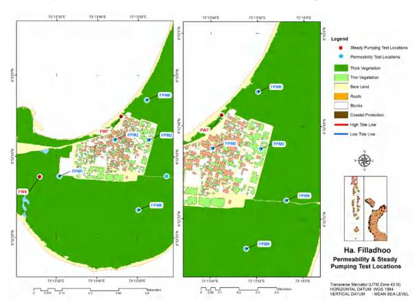
Figure 3-22: Locations of permeability and steady pumping tests in Filladhoo Island
