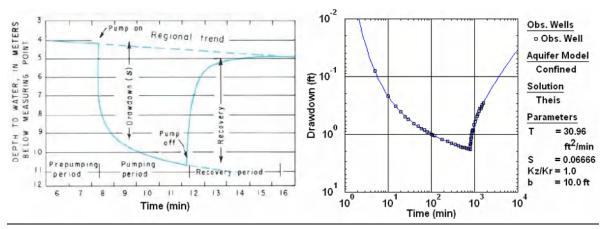
Figure 1-12: Typical well configuration for pumping recovery test in a confined aquifer and Estimation of aquifer properties by matching Theis (1935) type-curve solution to time-drawdown data
