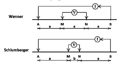
Figure 1-3: Electrode configurations -- Wenner and Schlumberger Arrays (Garofalo, 2014)
