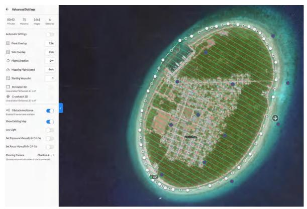
Figure 1-8: Example of a Flight Plan using Drone Deploy application and an example of spacing of Ground Control Points (GCPs) (red points) – Sh. Foakaidhoo Island.
